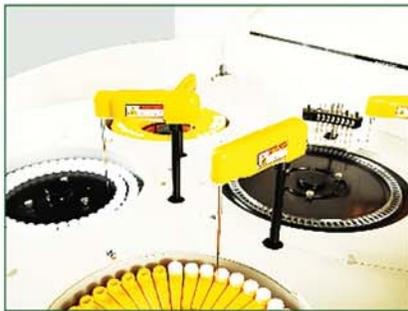
Sample probe / reagent probe with liquid level sensor, anti-collision sensor and automatic washing function.
